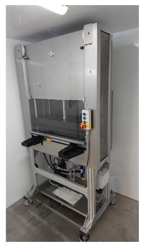
The Altracon Snow Compaction Unit is the unique machine to produce snow tracks with defined compression and repeatable conditions. Artificial or natural snow is compressed in the Snow Compaction Unit to produce a snow panel cartridge filled with snow or ice according to the parameters previously entered in the PC program. These cartridges fit for insertion into the HSLFT as snow track but may also be used in other testing devices.
