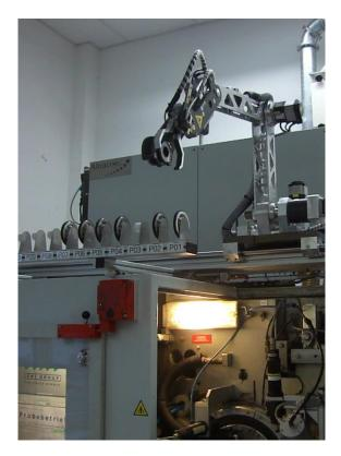
The Altracon GAL is a stationary loading unit, which extends the LAT100\* GROSCH wear testing system. It is supplementary mounted to the machine and allows **fully automated operation of the wear tests**.
