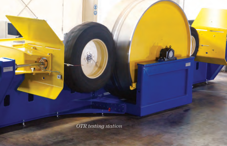
Foldable platform for ink-footprint application and plunger adaptation
