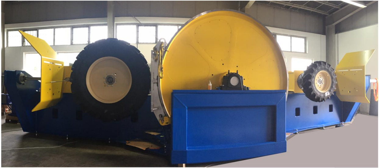
20 tons 2 Pos. Test machine for Agricultural Tires with tire footprint plate (left station)
