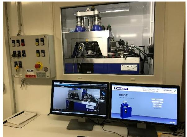
The activation may happen selectively with different signal wave forms with a defined number of cycles or also one-time activation with force- or stroke-control. The amount of cycles per test is limited under maximum conditions to keep the temperature of the rubber sample during the test on a constant level.
